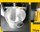
Rinse the tank and use a clean, dry stock pot to catch the hot water.
