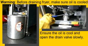
Remove the filter pan and position a stock pot under the drain.
